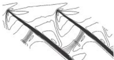
Figure 6. Mach Number Contours for Back Pressure Slightly Below the Maximum Choked Value.
