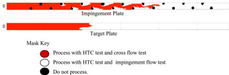
Fig. 8 Mask showing combination of tests used to calculate the heat transfer coefficient and effectiveness in different regions of the model
