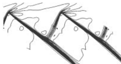
Figure 4. Mach Number Contours Near Stall in a Transonic Fan.
