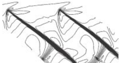
Figure 7. Mach Number Contours for Lowest Back Pressure Operating Point.
