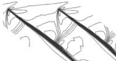
Figure 5. Mach Number Contours Near Peak Efficiency in a Transonic Fan.
