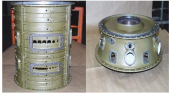
Fig. 5 Compressor casing coated with Sermatel 6F-1
